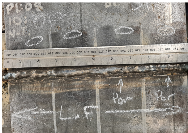
Figura 5.4: Weld 067 Lack of fusion.
