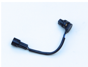
Figura 14: Sensor CMP de Yamaha R6
