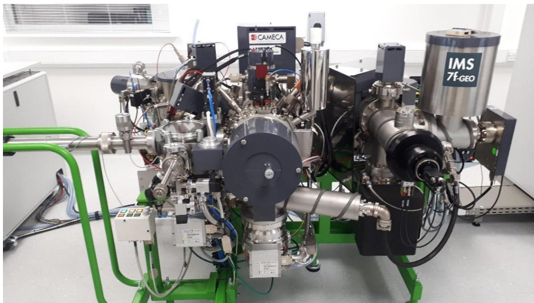
Figura 4.7: Microsonda Ionica, Cameca IMS 7f-Geo, en el en el Great Institute, School of Geosciences, University of Edinburgh.
