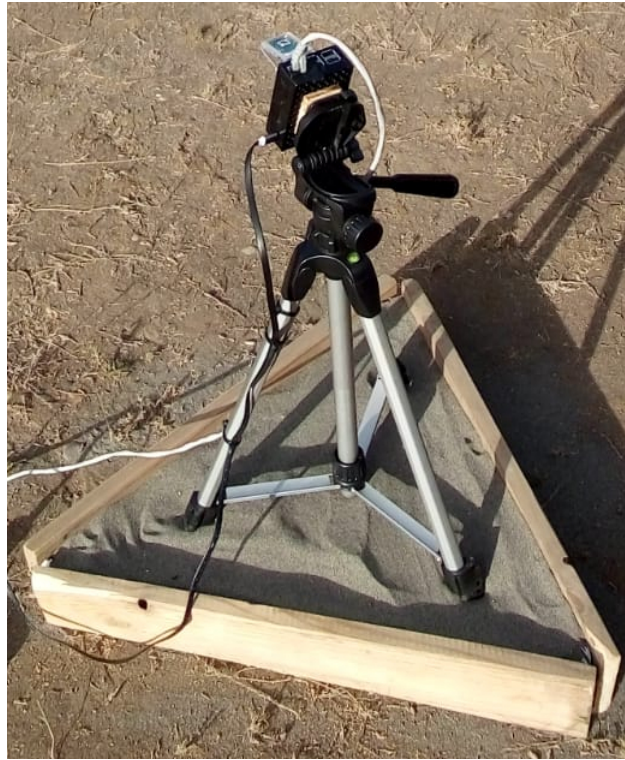
Figure 4.2: Equipment used for night sky measurements. This image shows the tripod, the black enclosure of the Raspberry Pi, and the transparent enclosure of the camera. The measurements were taken at 33^{\circ}00'48''\text{S} 70^{\circ}54'08''\text{W} on August 6th, 2016, and at 34^{\circ}25'42''\text{S} 70^{\circ}49'22''\text{W} on February 6th, 2017. Both measurements were made from 22:00 to 05:00 hours, local time (CLT).
