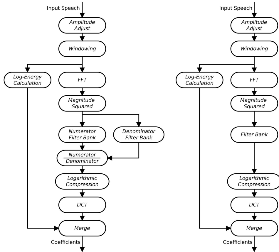
Figure 6: Flowcharts for LNCC (left) and MFCC (right) feature extraction: note the similarity between the two, with the only difference being the normalization of the filterbank outputs in LNCC . It is common to append delta and delta-delta co-efficients; this is not shown in the diagrams.
