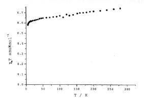
Fig.2. Temperature dependence of molar magnetic susceptibility of complex 1
