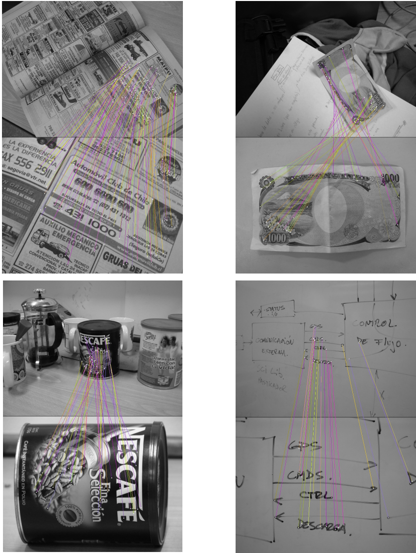
Fig. 1. Some examples of object recognition results that can be obtained with the new probabilistic model for hypothesis rejection
