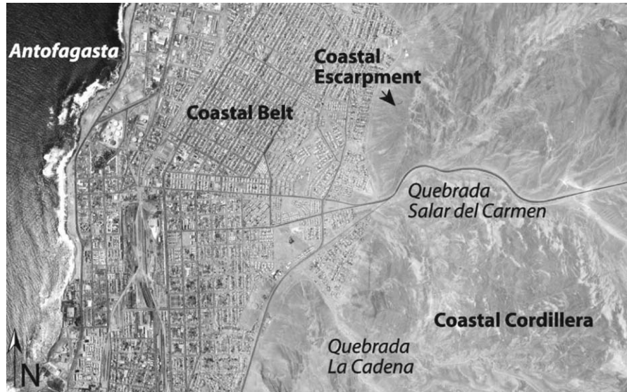
Fig. 3. Aerial photograph of Antofagasta in the discharge area of the Salar del Carmen and La Cadena Ravines (location in Fig. 2). This area was the most strongly affected by the debris flows during the 18 June 1991 event. According to Vargas et al. (2000), most of the city is located over Holocene alluvial fans.
