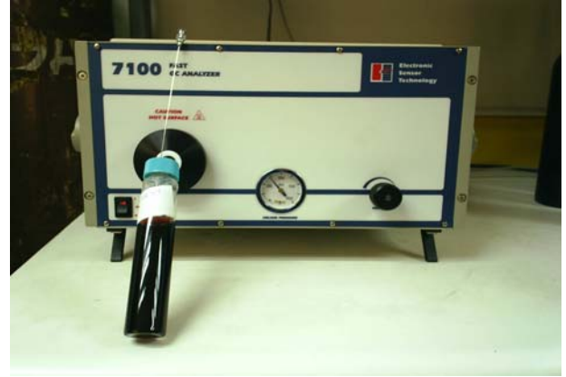
Fig. 4 Electronic nose model Fast GC Analyzer 7100 from Electronic Sensor Technology
