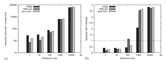
Figure 18. Readers and writers on four CPUs: (a) execution time with 1 thread and (b) speedup with four threads.
