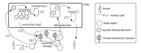
Figure 1. Operational sketch of a parallel object monitor.
