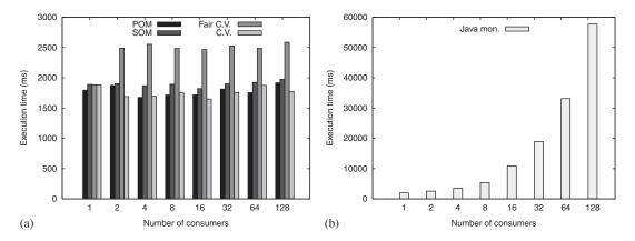
Figure 17. One producer/multiple consumers, buffer size 1, on four CPUs.
