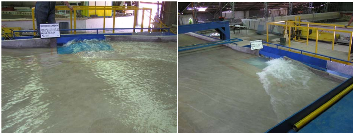
Figura 9.- Caso F: Izq. ( P_L=0.1\% ; P_T=3\% ; Q_T=120[\text{lt/s}] ) – Der. ( P_L=3\% ; P_T=2\% ; Q_T=180[\text{lt/s}] )
