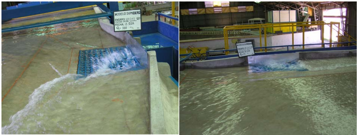
Figura 8.- Caso E: Izq. ( P_L=0.1\% ; P_T=1\% ; Q_T=180[\text{lt/s}] ) – Der. ( P_L=0.1\% ; P_T=3\% ; Q_T=120[\text{lt/s}] )
