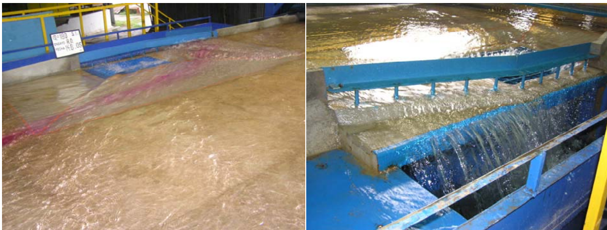
Figura 10.- Caso G: Izq. ( P_L=0.1\% ; P_T=3\% ; Q_T=180[\text{lt/s}] ) – Der. ( P_L=1\% ; P_T=1\% ; Q_T=120[\text{lt/s}] )
