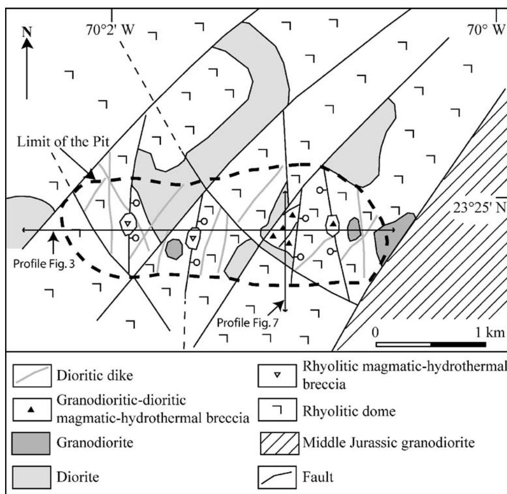
Fig. 2 Geological map of the Mantos Blancos ore deposit
