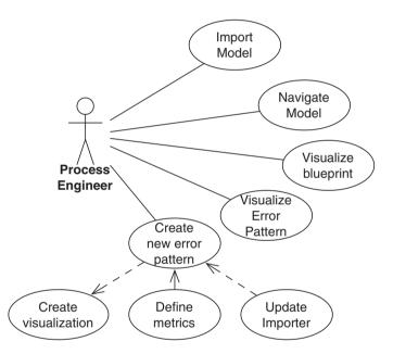
Figure 6. AVISPA use case diagram.
