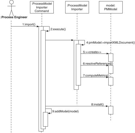
Figure 7. Importing an EPF process in AVISPA.
