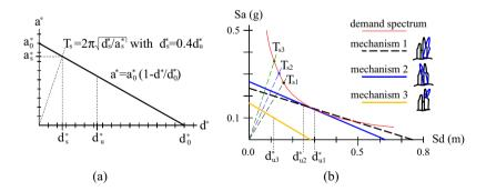
Fig. 19. Capacity spectrum: (a) definition and (b) computation for the considered collapse mechanisms.
