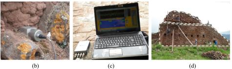
Fig. 3. OMA tests at Chokepukio: (a) test setup, (b) close up of a measurement node, (c) central acquisition station and (d) general view of the instrumented wall and the process of fixing sensors.
