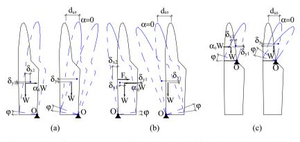
Fig. 18. Evolution of mechanisms: (a) 1st global rocking, (b) 2nd global rocking and (c) partial rocking.
