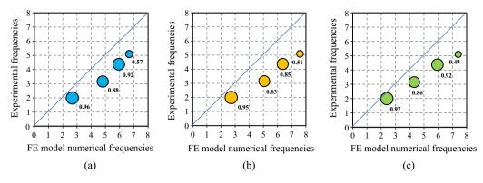
Fig. 8. FMAC graphics for: (a) Model 1, (b) Model 2 and (c) Model 3 (frequency values in Hz).
