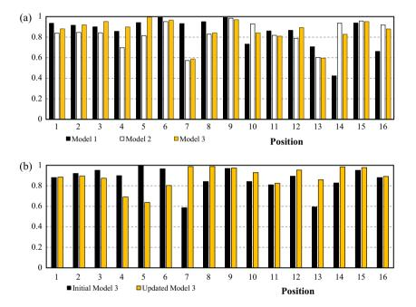
Fig. 9. Comparison of COMAC values for all the measured DOFs, between: (a) initial Models 1–3 and (b) initial and updated Model 3.
