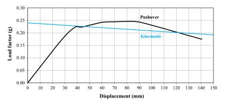
Fig. 16. Comparison of capacity curves obtained from the pushover and kinematic analyses.
