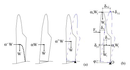
Fig. 14. Collapse mechanism for cantilever wall: (a) activation and (b) equilibrium variables.
