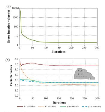
**Fig. 10.** Optimization process: (a) evolution of the objective function over iterations and (b) evolution of each variable over iterations.
