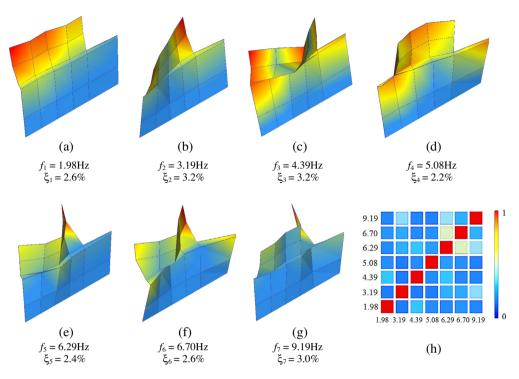
Fig. 6. Experimental mode shapes: (a-g) views of the first seven modes and (h) AutoMAC matrix.
