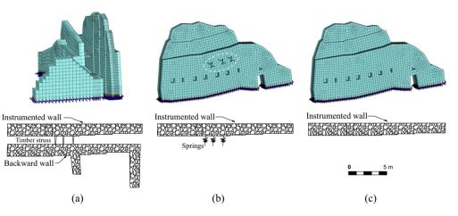
Fig. 7. Developed FE models: (a) Model 1 considering interaction between walls, (b) Model 2 assuming the instrumented wall as decoupled and (c) Model 3 considering only the instrumented wall.
