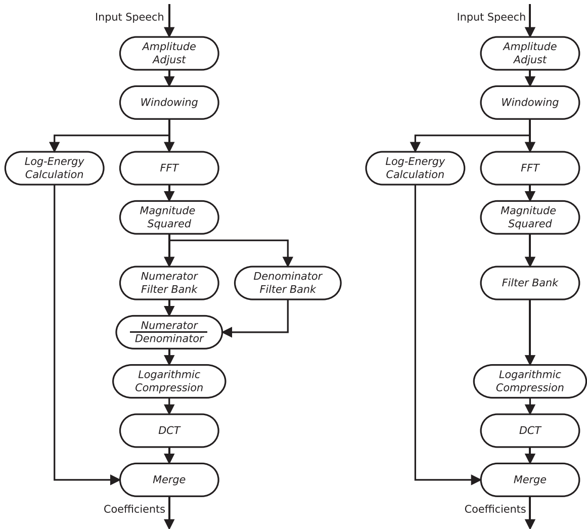
Fig. 6. Flowcharts for LNCC (left) and MFCC (right) feature extraction: note the similarity between the two, with the only difference being the normalization of the filterbank outputs in LNCC. It is common to append delta and delta-delta co-efficients; this is not shown in the diagrams.
