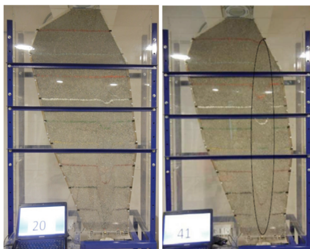
Figure 7—Isolated draw zone as measured during Experiment 1. at a) 33,280 ton for the drawpoint and at b) 68,224 (scaled values)
