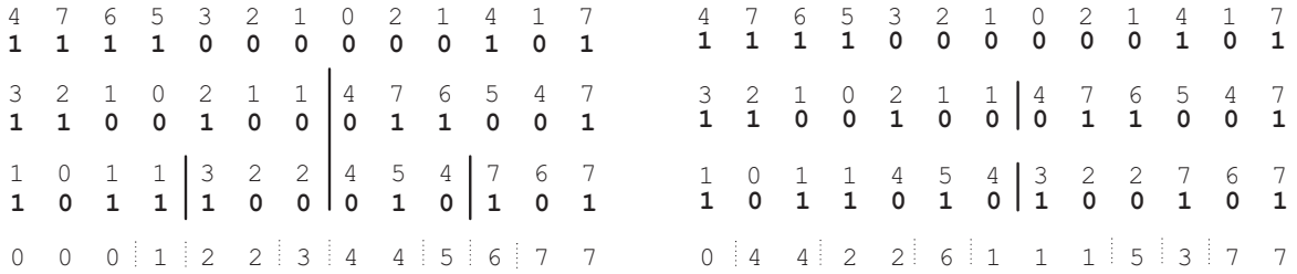
Fig. 4. On the left, the pointerless wavelet tree of Fig. 1. On the right, the wavelet matrix over the same sequence. One vertical line per level represents the position stored in the z_\ell values.
