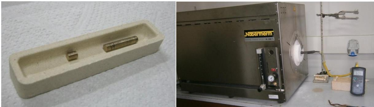
FIGURA 3-24: PORTA MUESTRAS CON LOS TROZOS A TRATAR Y CONTROL DE TEMPERATURA INTERNA DEL HORNO CON UNA TERMOCUPLA EXTERNA.
