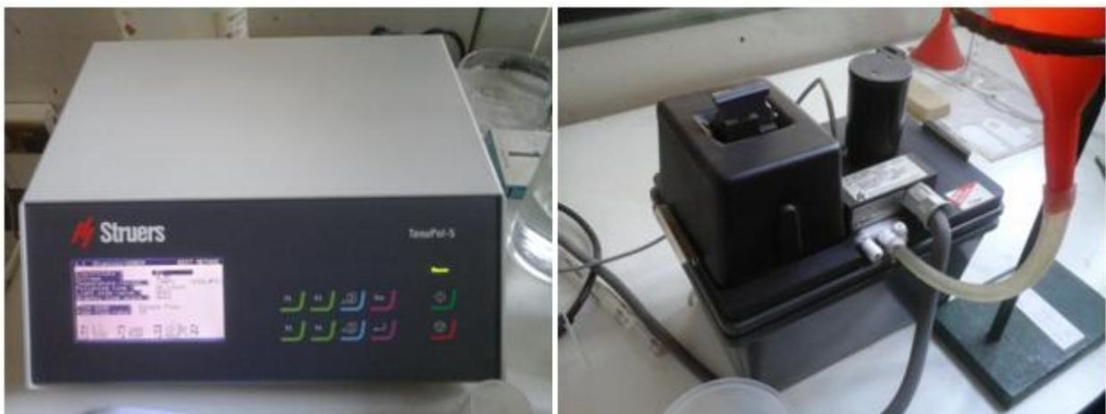
FIGURA 3-14: EQUIPO DE ELECTROPULIDO TENUPOL-5.
