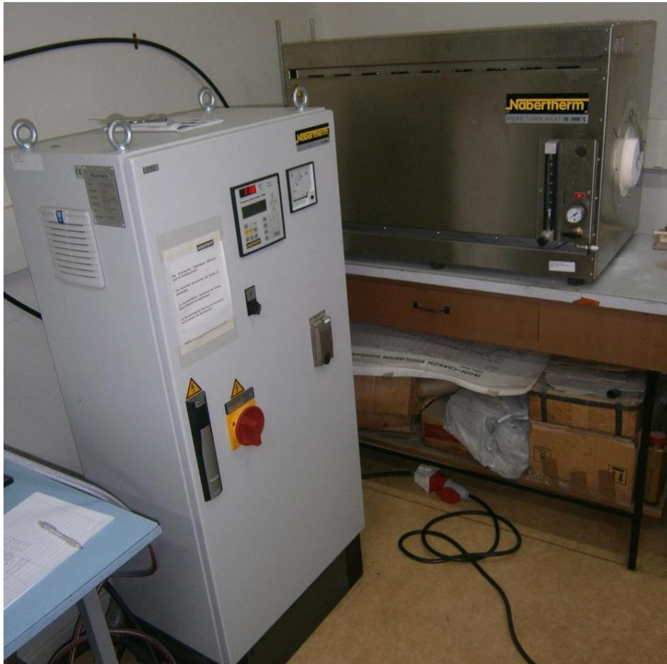
FIGURA 3-23: HORNO NABERTHERM 30-3000°C.
