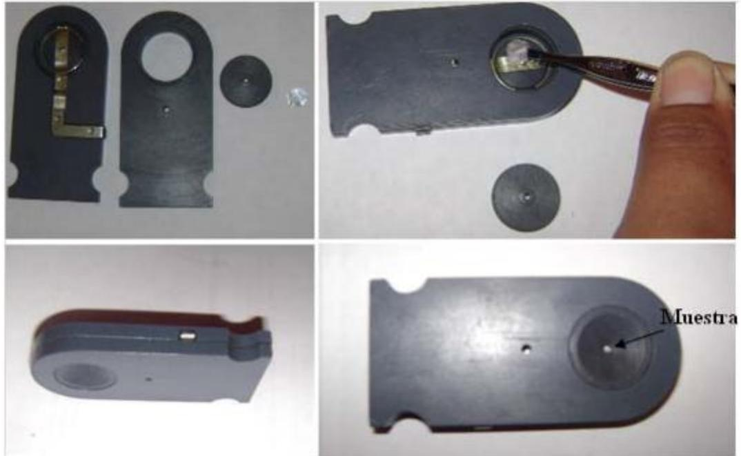
FIGURA 3-13: MONTAJE DE LÁMINAS AL PORTA MUESTRA.
