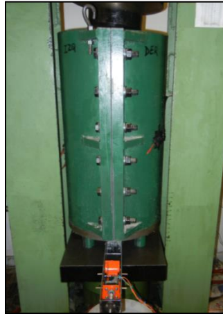
Figure 1: Cylindrical model in a press machine to apply different vertical loads, \sigma_v .
