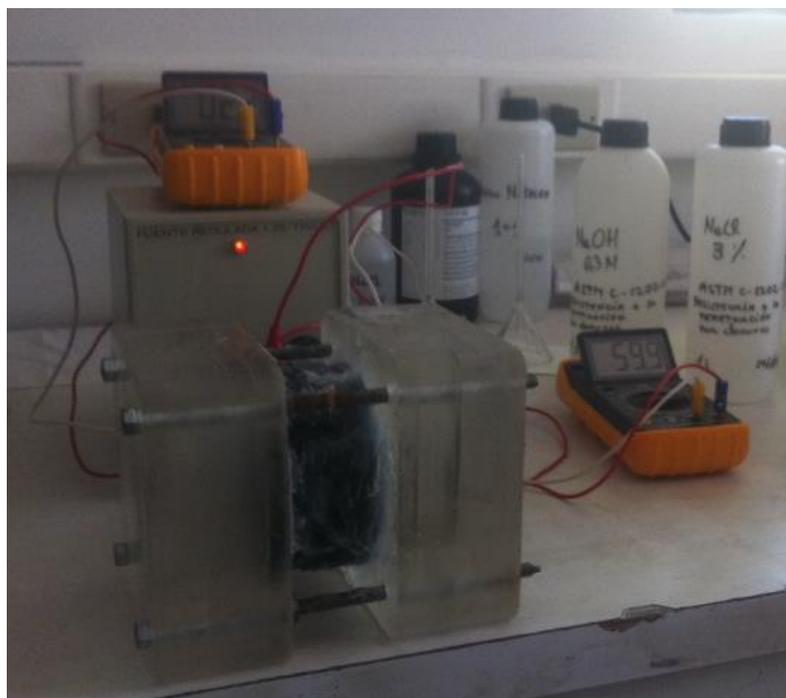
*Figura 12: Montaje experimental ASTM C 1202*
