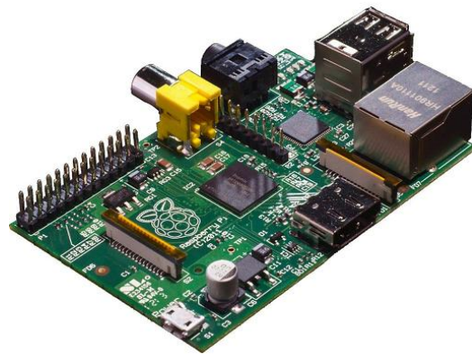
Figura 12: Raspberry Pi o Single Board Computer (SBC). Fuente: www.raspberrypi.org
