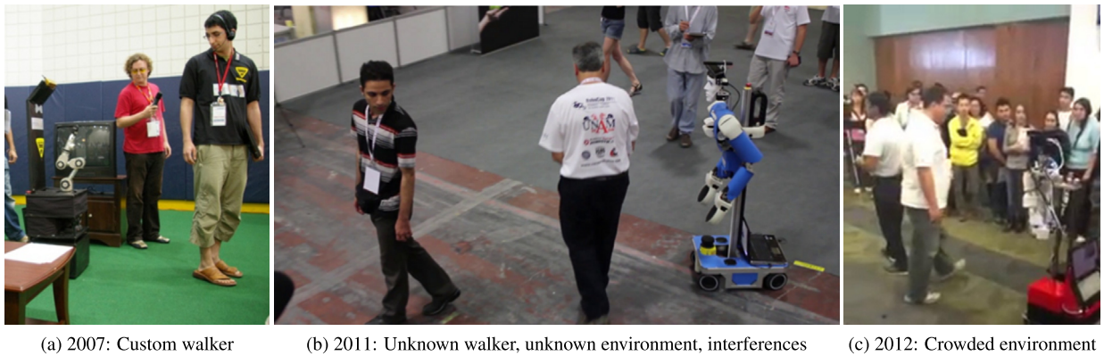
Fig. 2. Evolution of 'Follow me' test. Starting with known guides in a known environment, the test is now conducted with unknown guides in an unknown environment with several interferences along the route.
