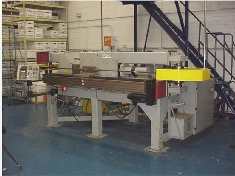
**Figura 3.4: WRI Medium Size Fatigue Testing Machine.**
