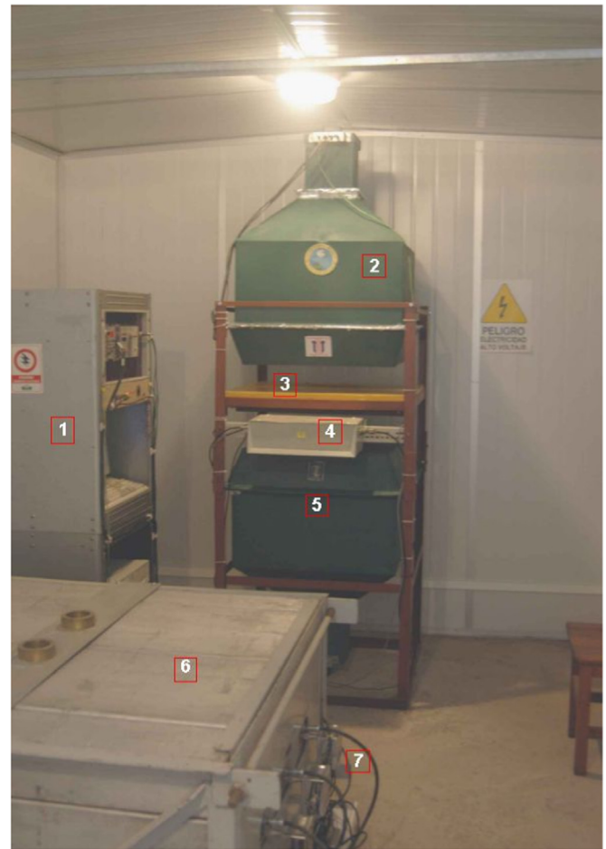
Fig. 3. Instruments details in PUTRE Observatory. Muon telescope 2-MMU. (1) Digital data systems for acquisition and data storage of Muon telescope and Neutron detectors. (2) Detector up in muon telescope constituted for phototube and plastic block in sealed pyramid metallic container, (3) Moderator, 0.05 m thick of Lead. (4) Distribution System of high and low voltage. (5) Detector down in muon telescope, constituted for plastic block in sealed pyramid metallic container and phototube (6) Neutron monitor 3IGYNM-3He Detectors, Lead and Polystyrene, (7) distribution System of high and low voltage. Collaboration UCH-UTA.
