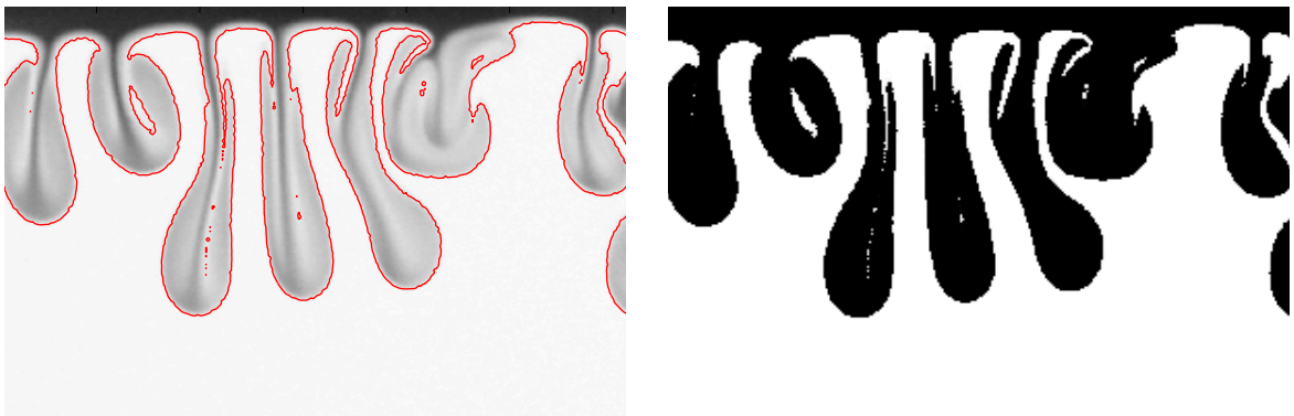
Figure 9.1.3: Example of Chan-Vese segmentation in an experimental image. We have lost much information about the mixing dynamics, if we only use one level set function. However, the edges are correctly segmented
