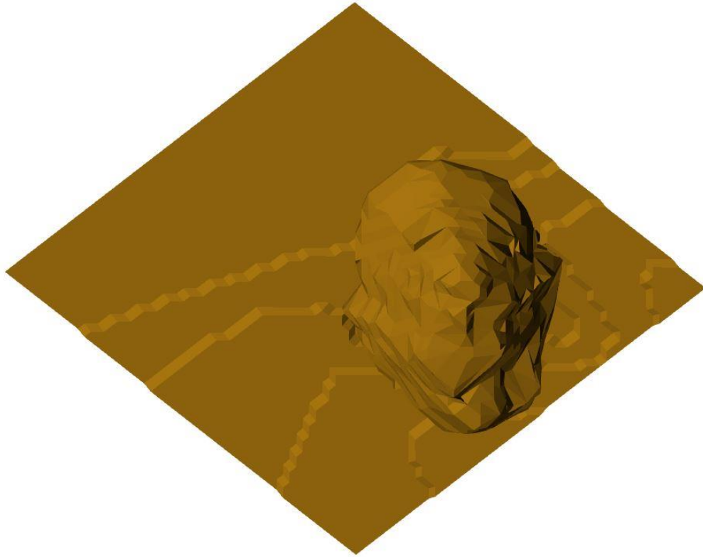
Figure 9.23: Excavation of pushback 3
