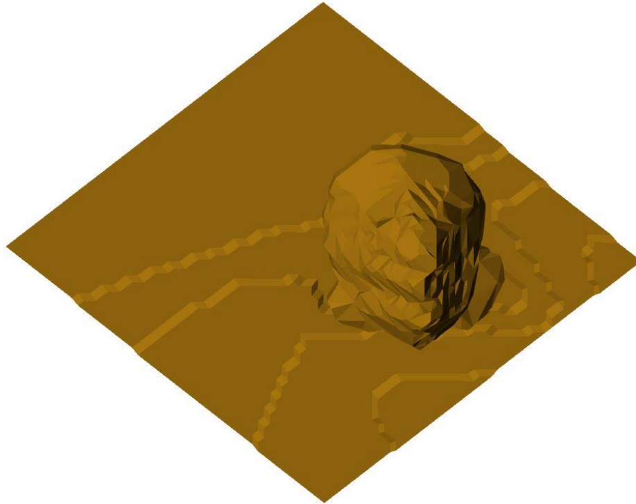
Figure 9.22: Excavation of pushback 2
