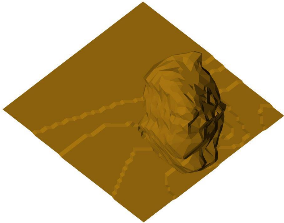
Figure 9.24: Excavation of pushback 4
