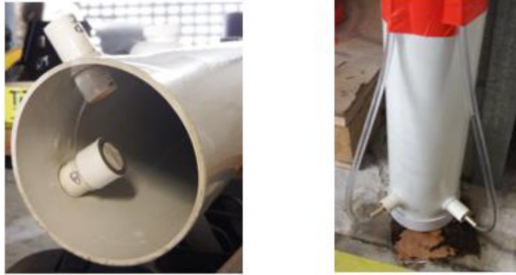
Figure 9.46: Porous filter test: two small PVC pipes (with and without filter) attached to a large PVC pipe
