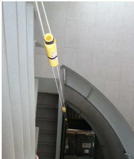
Figure 3.3: NSM array hanging from the stairs to test rope's resistance
