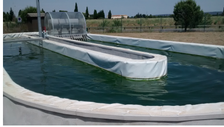
Figure 1.6. An open raceway pond is a photobioreactor with natural light (source Laboratoire de Biotechnologie de l'Environnement, INRA, Narbonne, France).
