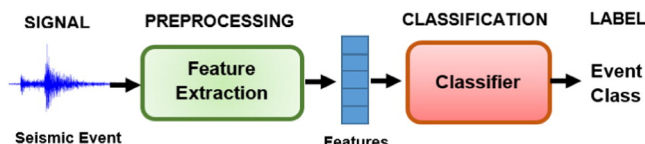
Fig. 4. General structure of the proposed pattern recognition system.
