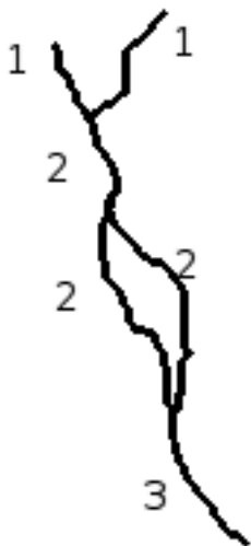
Figure 3: Example of incorrect Strahler order calculation in a braided stream. The order 2 stream splits into two substreams, which later merge and erroneously produce an order 3 stream according to the described algorithm. Braided streams in nature tend to split and merge many times throughout their path, which would induce many of these spurious Strahler order increments.
