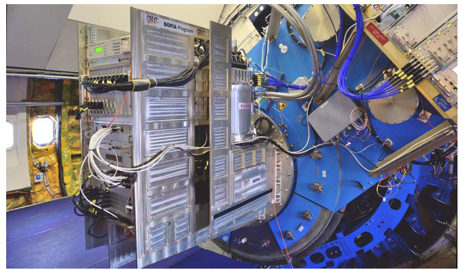
Fig. 18. GREAT/upGREAT instrument mounted on the Nasmyth tube of the SOFIA telescope. On the left side, the electronics rack houses the sensitive bias electronics, reference synthesizers and other motor controllers. The LFA cryostat can be partly seen on the right hand side of the central instrument structure. The pressurized helium hoses can be seen going from the rotary valve on the cryostat to the top part. Fifteen coaxial blue lines (14 for the LFA receiver and 1 for the L1 receiver) connect the cryostats IF outputs to the IF processors and spectrometers FFTS-4G.
