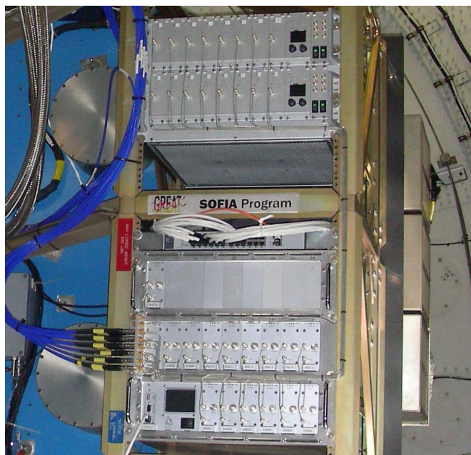
Fig. 12. upGREAT IF processor, located in the lower half, contains up to 22 cartridges. Each of them is amplifying, filtering, equalizing, and performing remote control leveling of its IF power to provide the nominal input power to the spectrometers. The upper half of the picture shows the FFTS-4G spectrometers. In this case 16 boards are installed.
