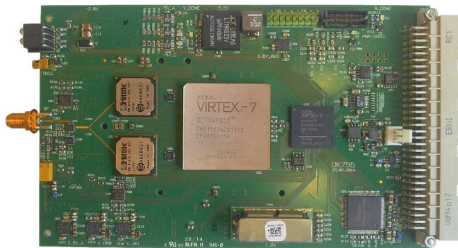
Fig. 13. FFTS-4G boards, using the VIRTEX-7 FPGA, two Hittite ADCs with 6-GHz input bandwidth are interleaved. Each board is capable of instantaneously sampling the 0–4 GHz band with up to 64 K spectral channels. For the upGREAT receivers, the number of channels is 32 K.
