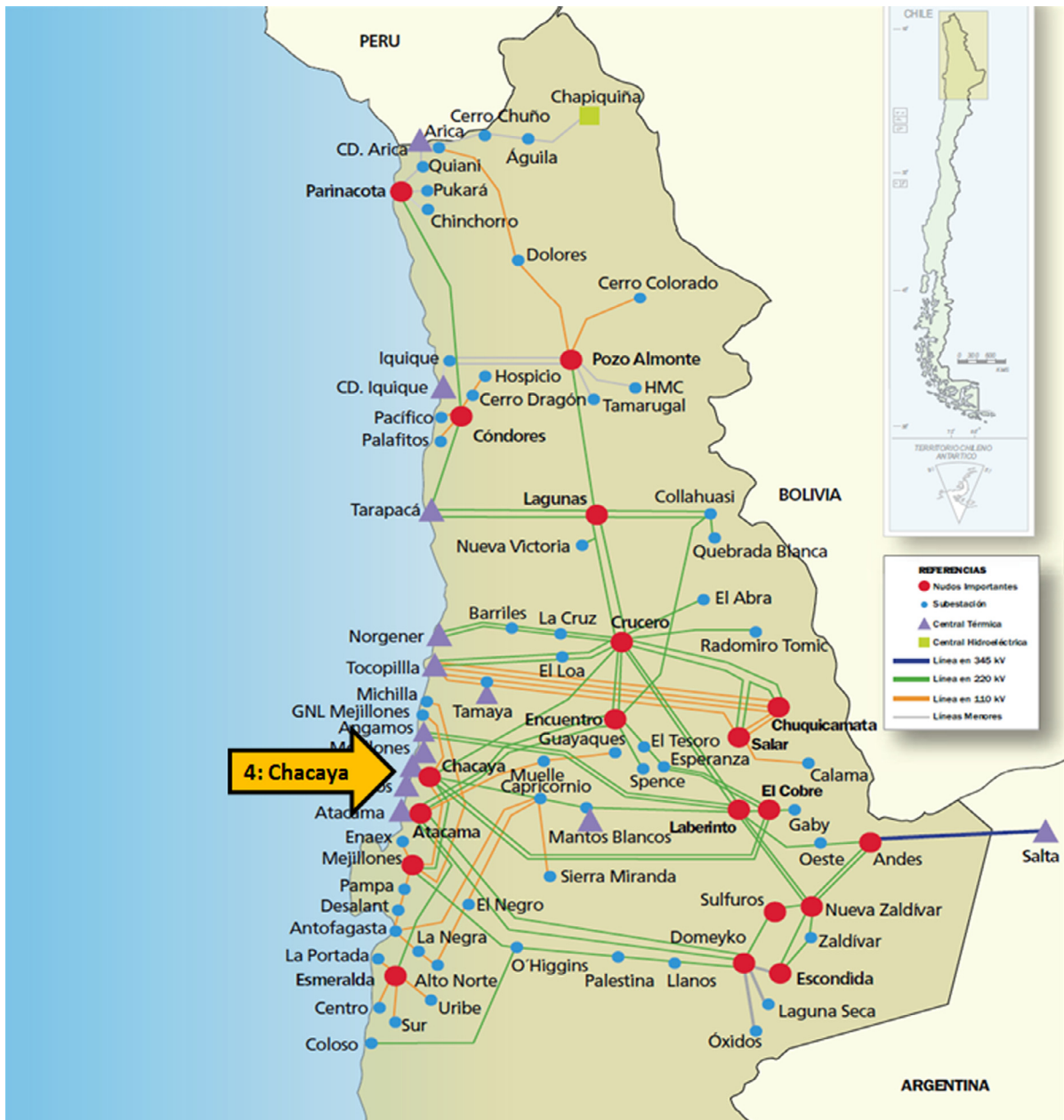
Fig. 3. Electrical and geographical location of the busbar chosen as injection point of wind power.
