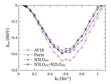
FIG. 3. Di-neutron binding energy in pure neutron matter as a function of Fermi momentum. Circles, asterisks, diamonds, and squares correspond to AV18, Paris, N3LO<sub>2N</sub>, and N3LO<sub>2N</sub> + N2LO<sub>3N</sub> bare potentials, respectively. Results correspond to pairs with zero total momentum.
