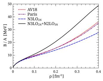
FIG. 9. Binding energy per neutron for pure neutronic matter as a function of density. Short-dashed, dash-dotted, dashed, and solid curves correspond to AV18, Paris, N3LO<sub>2N</sub>, and N3LO<sub>2N</sub> + N2LO<sub>3N</sub> bare potentials, respectively.
