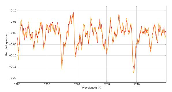
Fig. 6. Rectified spectra of GJ65 A (orange) and B (red), before Doppler-shift recentering. The vertical scale is the relative deviation in flux with respect to the moving median of each spectrum over a 5 Å window.
