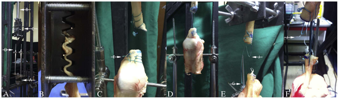
Fig. 3. Experimental set-up. A) Custom traction machine: white arrow A indicates the load cell device employed; white arrow B indicates the linear actuator; white arrow C indicates the compressive clamp; and white arrow D indicates the fixation site for the distal end of specimens. B) Compressive clamp at the tendon end. C) Krackow group specimen after biomechanical testing: white arrow E indicates suture rupture. D) Double-Kessler group specimen. E) Double-Dresden group specimen: white arrow G indicates the first suture rupture, and white arrow J indicates non-rupture of the second suture, generating a distal tear at the tendon end. F) Triple-Dresden group specimen: white arrow J indicates a tear pattern after biomechanical tests.
