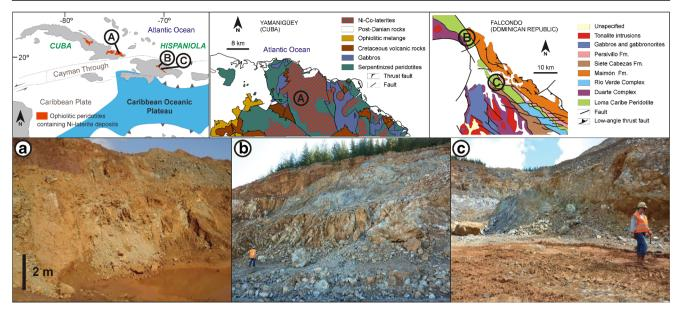
Fig. 1 Location of the Ni-laterite deposits studied in the Caribbean, schematic geological maps and field photographs depicting the mining pits of Yamanigüey, in Cuba (a), and Loma Caribe (b) and Loma Ortega (c) in the Dominican Republic
