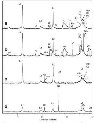
**Fig. 2** Powder X-ray diffractograms of saprolite from Yamanigüey (**a**), Loma Ortega (**b**), and Loma Caribe (**c**, **d**). Mineral abbreviations from Whitney and Evans (2010)
