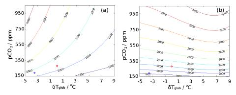
**Figure 3.** Steady-state land biomass (Gt C) as a function of global mean temperature (°C) and pCO<sub>2</sub> (ppm) deviations from the calibrated PI value for (a) the old uniform biosphere scheme and (b) the new biosphere scheme with three vegetation zones. The red circles denote PI and the blue circles LGM conditions.
