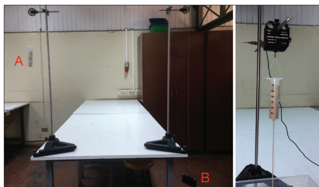
Fig. 1. Left: Experimental setup of the variable mass Atwood's machine. Right: Discharging flow of sand experimental setup. A PASCO Force Sensor was positioned at the top to collect the data.
