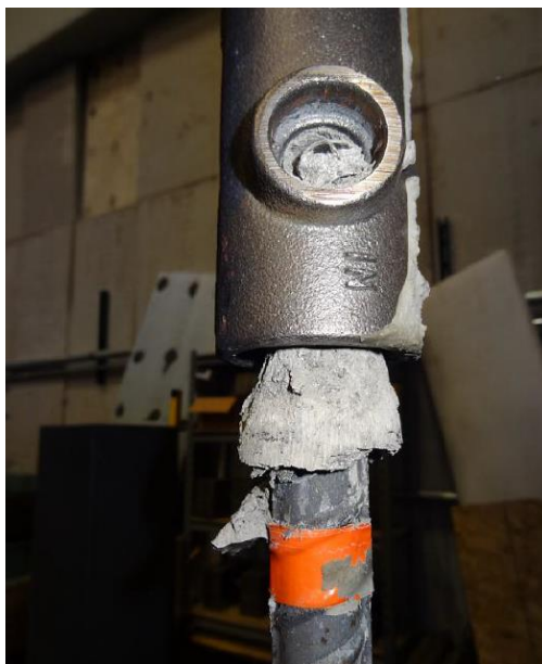
Figura 25: Falla pull out - lado ancho del conector. (Ref. 5)
