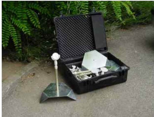
FIGURE 4.3: Riegl Retroreflector targets
