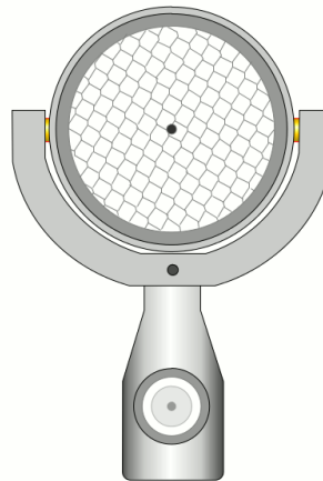
FIGURE 4.4: Riegl Retroreflector targets (schematic)
