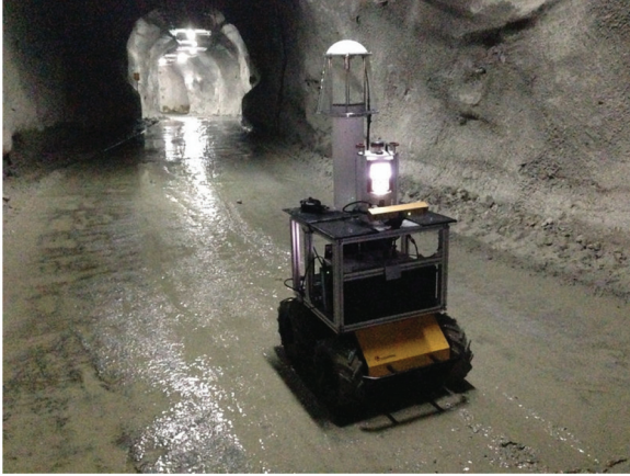
Fig. 1. The Husky A200 robot platform carrying a stereo camera, 3D lidar, and a radar, as it traverses through a tunnel in the copper mine for dataset collection.
