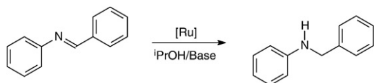
Scheme 1. Hydrogenation of N-benzylideneaniline by a new ruthenium (II) complex derived from polypyridine ligands.
