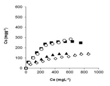
**Fig. 2.** Adsorption curves of Captan in natural soils (without incubation): ■:DIG-Captan, ▲ THL-Captan, ◯ HGS-Captan, ◇ MAO-Captan
