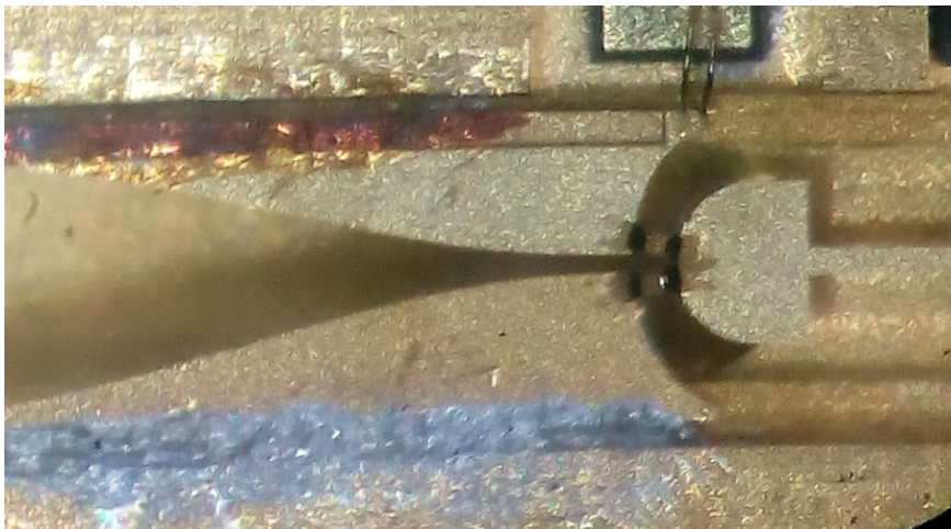
Figure 2.6: Balanced mixer with a fin-line transition to form a 180 degrees hybrid.
