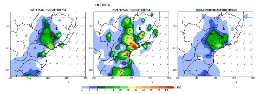
Percentage difference among monthly average CO, NOx and  $O_3$  mixing ratios in peak hours for the month of October, simulated by the experiments CONTROL and SA-INV on the 80km grid, and the average monthly near-surface wind field in m/s.
