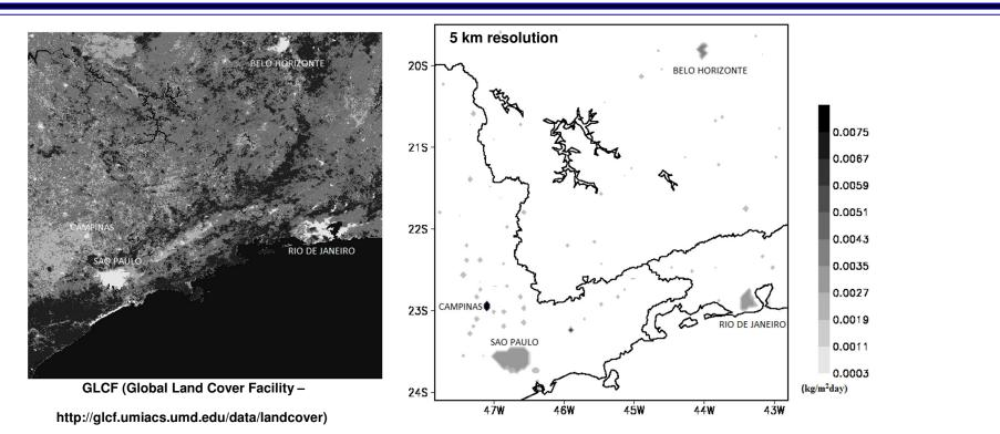
A new scheme is proposed in which urban areas are identified with a numerical algorithm based on Graham (1972), which identifies points pertaining to a pre-defined range of values, making a sweep from a central point generally defined as the center of the urban area.
