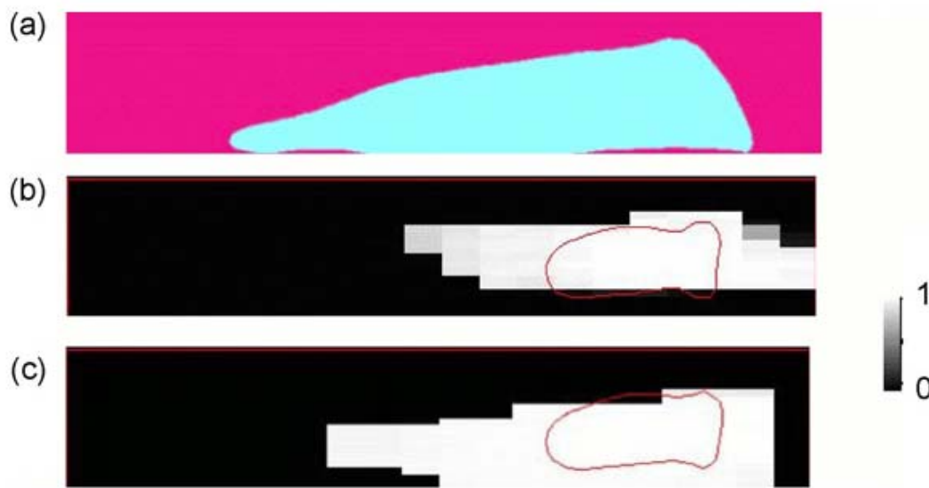
Figure 2.30: Comparison between a conceptual geological model and inversion results. (a) Conceptual model. (b) Probability to obtain the unit after inversion of the gravity field only. (c) Probability to obtain the unit after simultaneous inversion of the gravity field and the five tensors components (Guillen et al., 2008)
