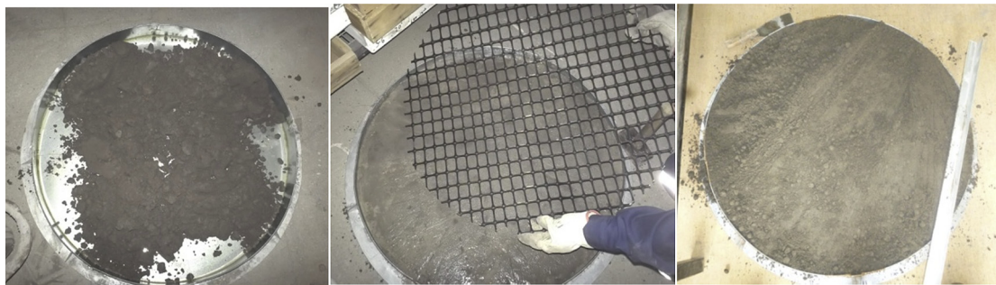
Fig. 6. Fabrication of test specimen with geogrid.
