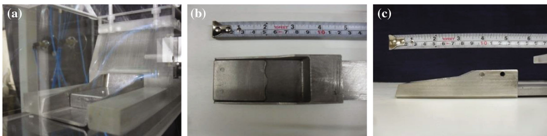
Fig. 1 Dozer feeder system at reduced scale. a Isometric view at the draw point, b plan view, and c lateral view
