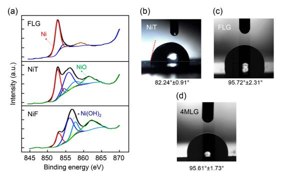
**Figure 2.** Surface composition and hidrophobicity of coated and uncoted Ni samples. (**a**) XPS Ni  $2p_{3/2}$  spectra of coated and uncoated Ni, including peak fitting to identify Ni (red, yellow and orange), NiO (green) and Ni(OH)<sub>2</sub> (blue) contributions. This allows the identification of FLG control sample (NiT). Images of contact angle measurements using Milli-Q water in contact with (**b**) NiT; (**c**) FLG and (**d**) 4MLG.
