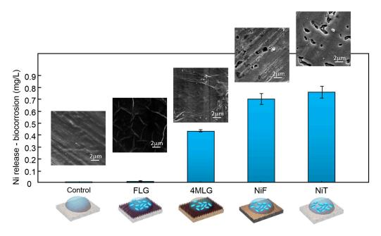
**Figure 4.** Ni ion release from graphene-coated and uncoated Ni samples. ICP measurements on coated and uncoated Ni samples after 24 h of bacteria contact showing Ni dissolution. Dissolved Ni for graphene-coated Ni samples in contact with bacteria (*E. coli*) is below technique's detection limit, as well as control sample. NiT and NiF in contact with bacteria present high nickel ion release. SEM images show morphology of samples after bacterial exposure.
