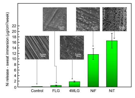
**Figure 5.** Ni ion release from graphene-coated samples exposed to artificial sweat. ICP measurements on grown and transferred graphene-coated and uncoated Ni samples after 1 week of sweat immersion showing Ni dissolution. Uncoated samples (NiT and NiF) in contact with sweat present highest Ni ion release. All samples where 1 cm<sup>2</sup>. SEM images show morphology of samples after sweat exposure.
