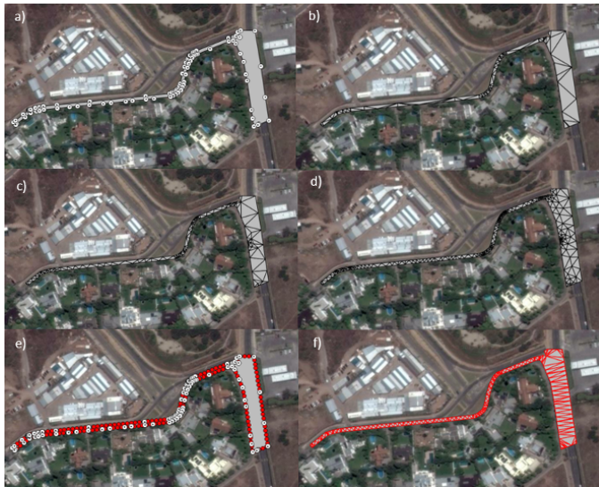
Figure 5.31. a) HRU associated with a road segment with the original nodes. b) Triangulation without restriction. c) Triangulation with restriction on the maximum area of 200 \text{ m}^2 . d) Triangulation with restriction on the minimum angle of 30^\circ . e) HRU where nodes are separated with a maximum distance of 5 m (f) and its triangulation without restriction on the area or on the angles. For a color version of the figure, see www.iste.co.uk/baghdadi/qgis4.zip
