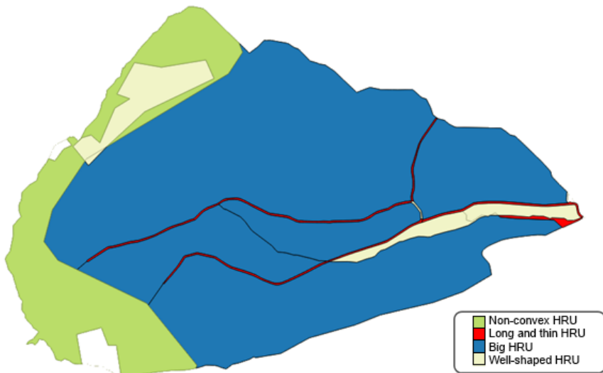
Figure 5.4. Badly-shaped elements in the Mercier subcatchment. For a color version of the figure, see www.iste.co.uk/baghdadi/qgis4.zip
