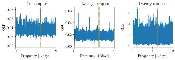
Figure 5. Average QMI across five bands for the example shown in Figure 4. In both cases the true period is correctly detected. For reference we include the multiband LS periodogram for the 20-sample case.
