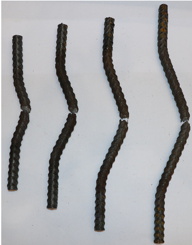
Fig. 5. Fatigue failure of buckled reinforcing bars with different slenderness ratio.
